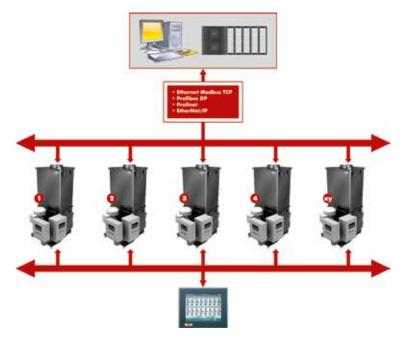
Multiple feeder control solution for gravimetric feeders with feeder mounted control modules for direct connection to a host/PLC system (optionally available with control cabinet mounted control modules)
