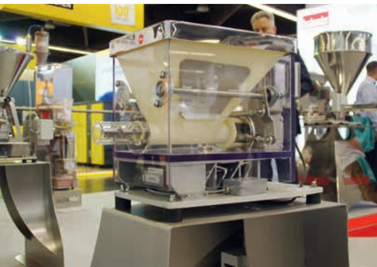
The transparent FlexWall shows its massage paddles.
