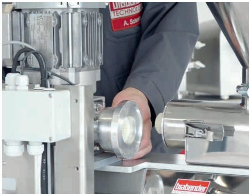
In the extended version, the motor remains on the unit and is only moved for disassembly, so that the screw can be pulled from the rear.
