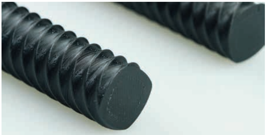
New quadruple-flight screws were designed on customer's demand.
