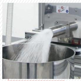
Img. 4: Vented air pushes ingredient out in the event of a blocked filter
