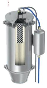
with a pulse of compressed air that blows trapped ingredient back into the process. In a continuous process, jet filter cleaning occurs at the end of the refill during the material stabilization phase without interfering with the gravimetric cycle. When very expensive or toxic materials are involved, a jet filter is a must, but it can also be a good option for other powders and fine pellets. "The best onstration in the Technical Center showing
