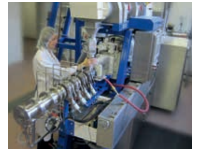
Clextral uses twin screw extrusion to produce a new generation of meat substitute.
