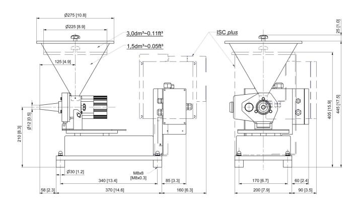
Weight with 1.5 dm $^3$ /0.05 ft $^3$  extension hopper approx. 20 kg (44.1 lb) Weight with 3.0 dm $^3$ /0.11 ft $^3$  extension hopper approx. 21 kg (46.3 lb)
